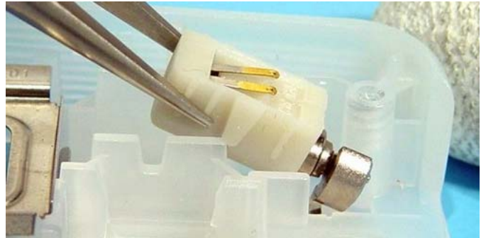
If you need to change the Vibra Motor, strong tweezers or pliers can be taken.
