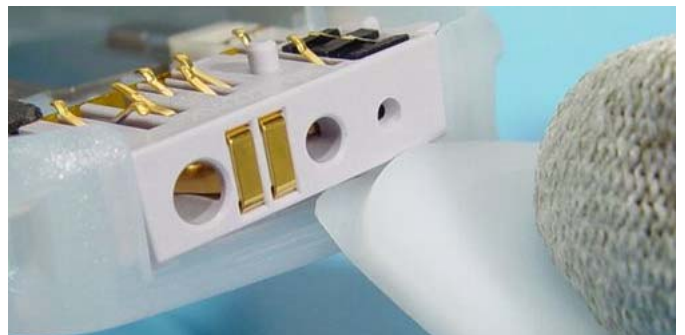
To loosen the System Connector you can use SRT-6 opening tool. Take care not to scratch the D-Cover or the connector housing.
