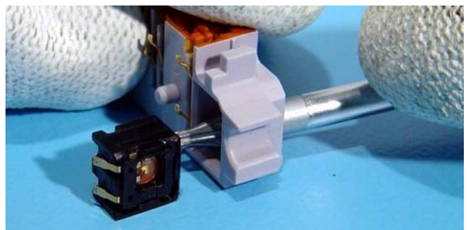
When re-assembling the Microphone remember the right direction. The hole of the Microphone has to point to the hole of the connector housing.
