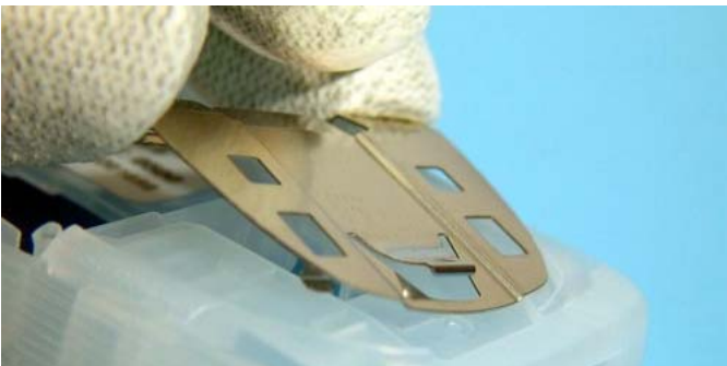
After releasing the two hooks, you can remove the Release Spring easily.
